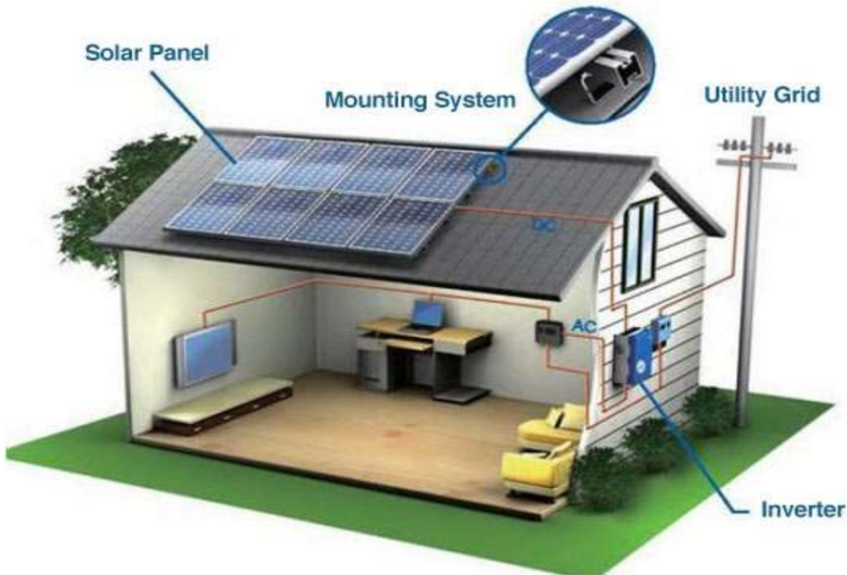
EXAMPLE OF GRID-TIED SYSTEM (Connected directly to utility grid, no battery storage)
